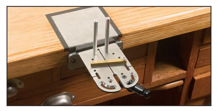
The Knew Concepts Bench Pin has been designed from the ground up for piercing and bench work. It is machined from a solid 3/16" slab of stainless steel. First, so that it is stiff and rigid enough to support your work without bouncing as you cut, yet remain thin enough not to interfere with your full stroke. This thinness is helpful when doing delicate piercing. Second, it is stainless steel so that even when you do cut it, it doesn't contaminate your sweeps.
