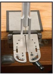
put the handpiece in front of the guideposts, you have no clearance at all, but that position is most useful for wax milling and other cutting tasks. It is also easier to leave the posts permanently attached if they're toward the rear, rather than the original front position. The choice is yours.
