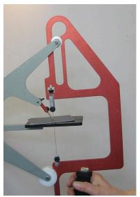
simultaneously sliding the blade through the slot of the bench pin.
